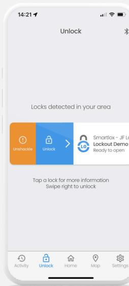
**Step 2:** Swipe right on the lock and select 'Unshackle' to release the shackle from the lock body.
